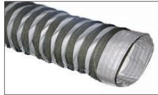
SPIRA- EXHAUST for extraction: with dense vacuum-resistant spiral, PVC (+100°C), CSM (+175°C), glass fabric (+800°C)
