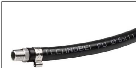
TECHNOBEL PU hose DN6 with fitted stainless steel (AISI 316) end with BSPT 1/8" male thread (NM-VT123-02). Mounted with an AISI 304 stainless steel EAR CLIP (AB-23012028).
