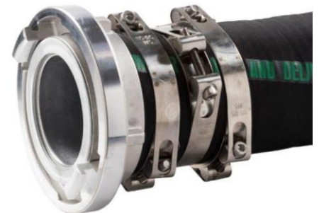
TORONTO LIGHT DN110 with tip STORZ in aluminium (catch distance 133 mm, ST-12-133110-11), twin-screw ties DPC version W5 in AISI 316 steel; 3 bands placed between the notches of the tip.
