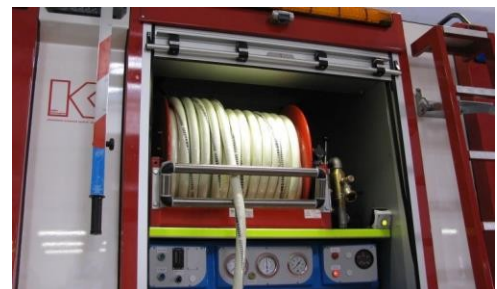
CHICAGO EN GL DN19 hose on a reel mounted on a fire engine.
