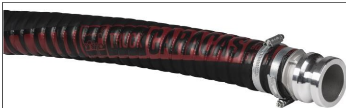
CARACAS hose DN51 with CAMLOCK E 2" aluminium coupling (AC-E-200-A) mounted with galvanised steel worm bands.
