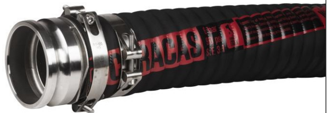
CARACAS hose DN102 with stainless steel (AISI 316) CAMLOCK E 4" coupling (AC-E-400-SS) mounted with strong AISI 316 stainless steel screw ties (AB-DPC-110-120-W5).
