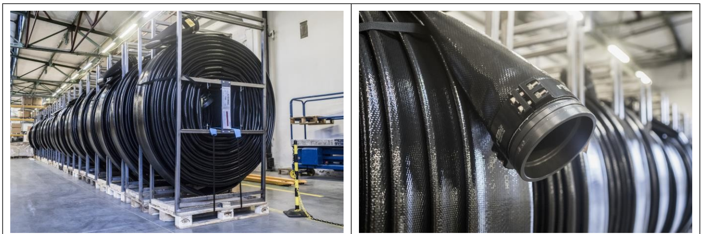
Flat hoses DN203 with grooved couplings mounted with special clamps, designed for the mine drainage system.
