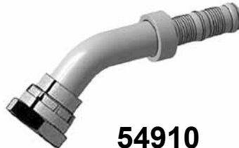
BURGACLIP - connection fitting with a female metric thread, type DIN 3865, 24° cone, light series
