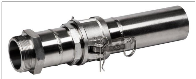
CAMLOCK connector socket butt-welded to seamless EN 10216-2 pipe (pipe index: MPR-RBSZ-060X2.9- SS321) in AISI 321 steel.
