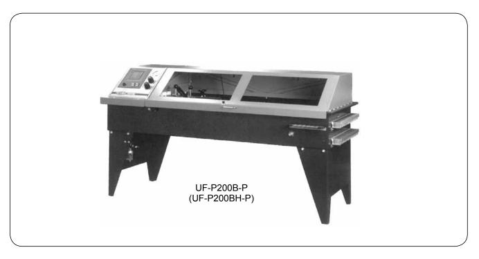
The test bench designed for testing hydraulic hose assemblies with static pressure. The machine used in series production plants allows to carry out final inspection of the quality of manufactured assemblies.
