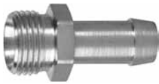
SA type fitting with metric male thread and hose tail (24° cone seal)
