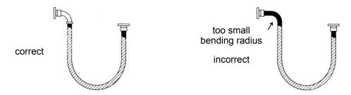
Bending radius of a steel hose should not be smaller than the one given in the manual to avoid material fatigue or premature damage. It is necessary to prevent sharp bends in the hose near its fittings.
