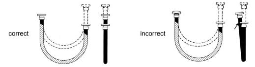
It is kinking of a hose that causes failure or premature wear. So as to prevent hose kinking a swivel flange should be installed on one of the hose ends. The hose should always be installed in such a way that its movement is the same as its symmetry axis.
