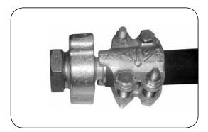
TUBES INTERNATIONAL® warns against using steam hoses with fittings assembled on a hose with a crimped ferrule. Such an assembly method does not allow to tighten it during operation. It is very important as during operation the elastic quality of hose material (rubber) is gradually decreasing. When a clamp cannot be tightened a leakage or even a catastrophic burst from the fitting of a hose can occur!
