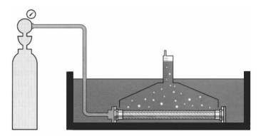
The rate of permeation is higher when the particles of gases are small (helium, hydrogen) and when the hose wall is thin and with porosity. For those reasons:
