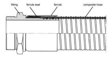
Due to their unique construction and complex assembly technology, the composite hoses are supplied as complete hose assemblies only.
